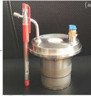
A miniaturized 2.45 GHz ECR ion source at Peking University, Wen Jia-Mei et.al.
