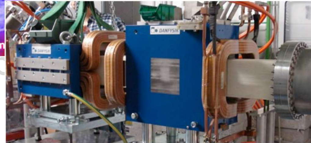
Fig. 11: Picture of the CNAO scanning dipoles for the horizontal beamline
