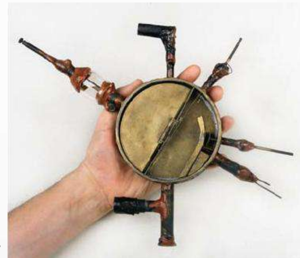
Livingstone cyclotron, diam. 10 cm. 80 keV protons
