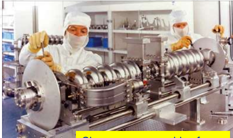
Clean room assembly of superconducting RF cavities
