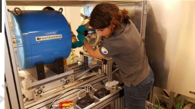
Supernanogan from Pantechnik 14.5 GHz ECR Ion Source installed at MedAustron
