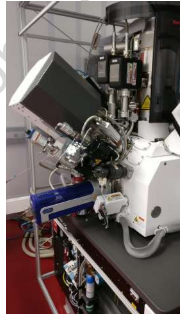
Xenon Focused Ion Source (FIB) at IST Austria, from ThermoFisher, Credit: S. Bagiante
