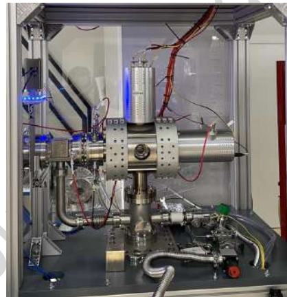
Electron Beam Ion Source Installed at TUWien Austria, Credit: R. Willhelm
