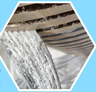
Superconducting coils with epoxy often exhibit "training," needing multiple quenches before reaching the nominal current. Recent tests show wax as a better alternative in stress-managed coils. A wax-impregnated Nb3Sn cable reached the short-sample limit without a single quench. (test performed by the Paul Scherrer Institute).
